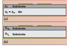
▲ Fig. 1 Cross-sectional views of a suspended coupled microstrip (a), and a composite laminate coupled microstrip (b).
