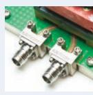
Southwest Microwave's high performance 1.85 mm end launch connector is now offered with a 5 mil diameter launch pin. This connector is designed to pro-
